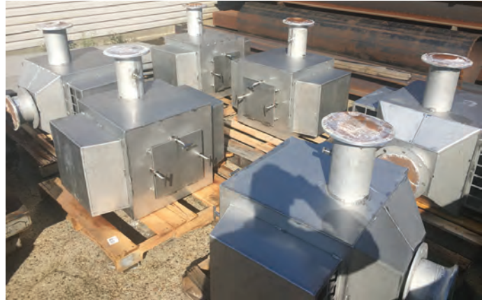
HC Storage Tank Vent Hoods
