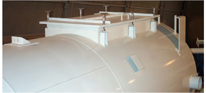
Vacuum System Filter Separator
