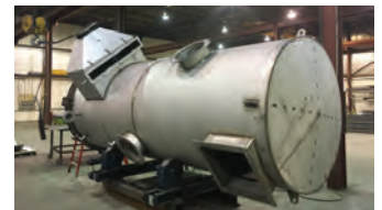
Mist Elimination Cooler Vessel
